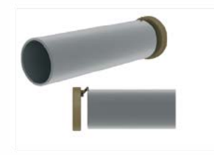
12. Grinding of weld at pipe ends and beveling
