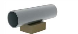
16. Magnetic particle and ultrasonic inspection of both pipe ends
