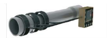
4. Magnetic particle inspection (MPI) of pipe end
