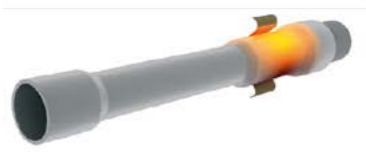
12. Heating and heat treatment of weld area
