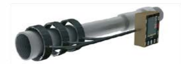
15. Flaw detecting of weld point
