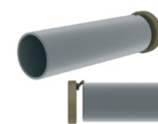
12. Grinding of weld at pipe ends and beveling
