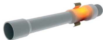
12. Heating and heat treatment of weld area
