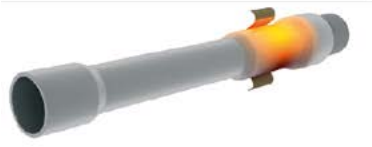
12. Heating and heat treatment of weld area
