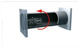
8. Internal pipe surface blast cleaning in Shot Blaster 2
