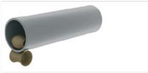
4. Post-bending of the longitudinal plate edges
