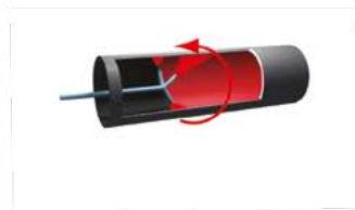
11. Coating application on pipes (in coating chamber)
