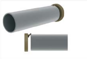
12. Grinding of weld at pipe ends and beveling
