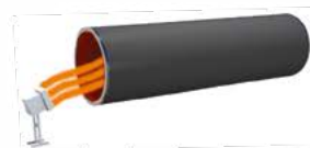
12. Internal coating pre-curing
