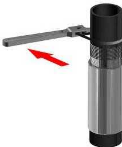
Figure 10 – Make-up start with strap tongs
