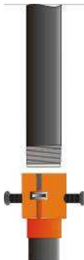
Figure 5 – Make-up with special bell guide
