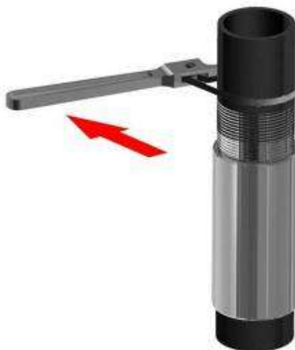
Figure 10 – Make-up start with strap tongs
