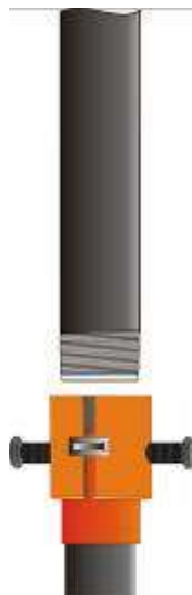
Figure 5 – Make-up with special bell guide
