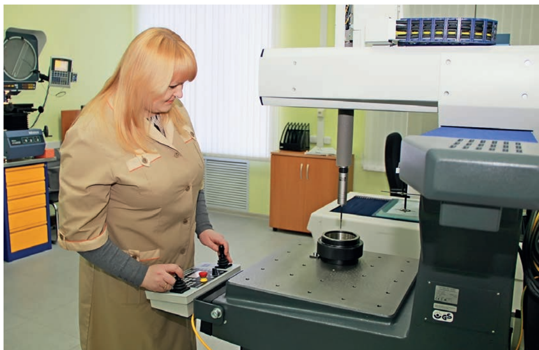
Verification of thread gauges in the metrological laboratory
