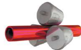
6 Shell rolling into pipes on Assel mills
