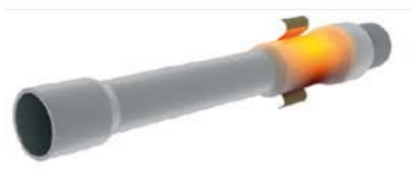
12. Heating and heat treatment of weld area
