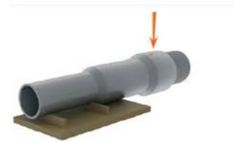
18. Paint pipe body and protection of treading
