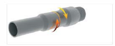
11. Friction welding of tool-joint to drill pipe
