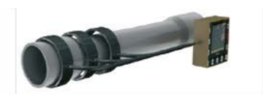
4. Magnetic particle inspection (MPI) of pipe end
