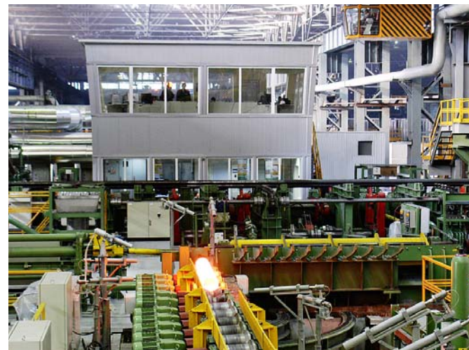
Premium Quality Finishing (PQF) seamless rolling mill at TAGMET
