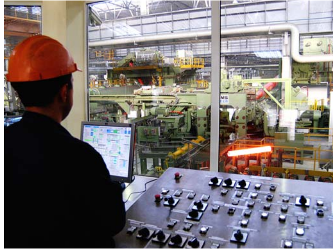
Operator's console at piercing mill at TAGMET
